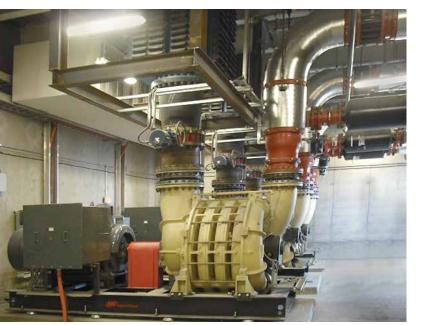
Mining Application Model 675.04 800 Hp, 3600 rpm 15000 scfm 7.25 psig
